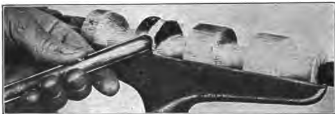
Fig. 53. Turning Bead with Gouge.
